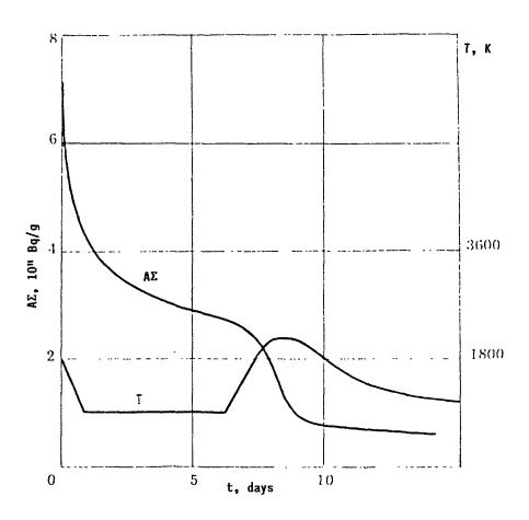
Fig. 5. Variation of activity and temperature of the fuel with time
