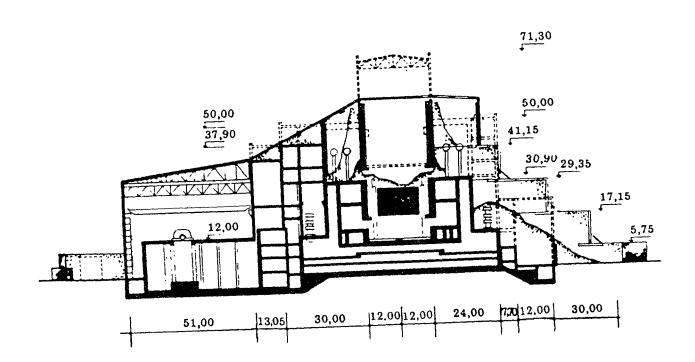
Fig. 7. Diagram showing one scheme for the isolation and encasement of unit 4 (vertical cross-section)
