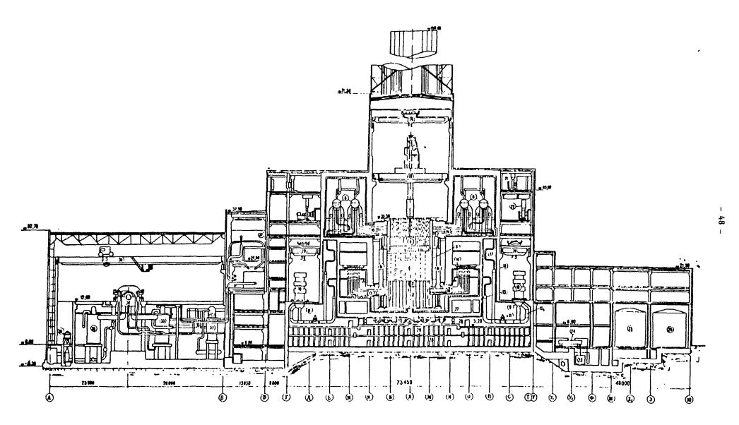
Fig. 1. Cross-section through the main structures of a power plant with an RBMK-1000 reactor (with localization zone)
