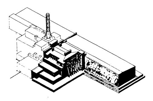
$\underline{\text{Fig. 8}}$ . General view of one scheme for the isolation and encasement of unit 4
