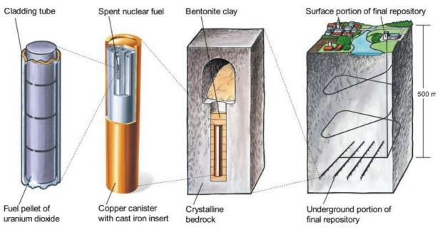
Figure 5. The Swedish concept for the disposal of spent nuclear fuel as an illustration of the multi-barrier concept.
