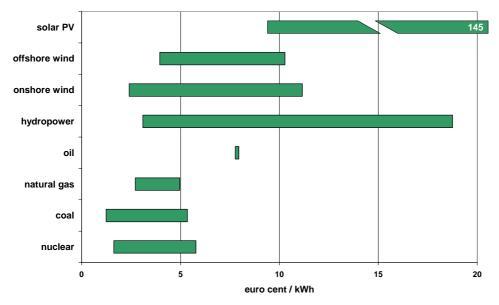
Figure A-3. The ranges of levelized costs associated with new construction as estimated in seven recent studies for electricity generating technologies in different countries. (PV = photovoltaic).
