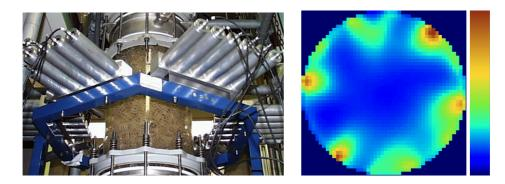
Figure E-1. A tomography system with 36 collimated detectors is installed around the column. The liquid phase, labeled with 1.9 GBq of technetium-99m, is injected, and the result shows some water channeling on the wall of the column.
