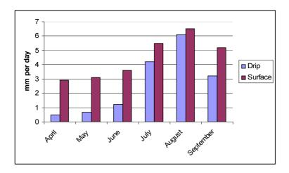
FIG. 1-6. Cotton grown in Syria: the daily irrigation requirement ( $mm \ day^{-1}$ ) is reported on a monthly basis for drip and surface irrigation. During the first three months of the cropping season, more than 60% of irrigation water can be saved using drip irrigation.
