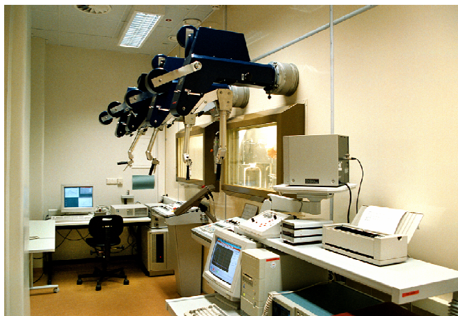
FIG. 2 Hot cells with manipulators used for radioisotopes/radiopharmaceuticals production available from commercial sources.
