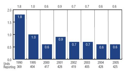
FIG. A-2. Unplanned scrams per 7000 hours critical. Source: WANO 2005 Performance Indicators.
