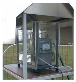
Fig. H-3: A high volume air sampler, for use in air pollution or radon monitoring
