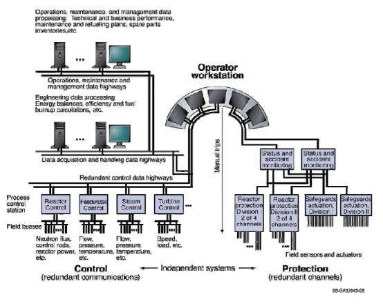
FIG.V-3. Typical I&C architecture for a plant with a digital I&C system for control and an analog I&C system for safety (labelled "protection" in the figure)<sup>2</sup>. (Source: US National Research Council).
