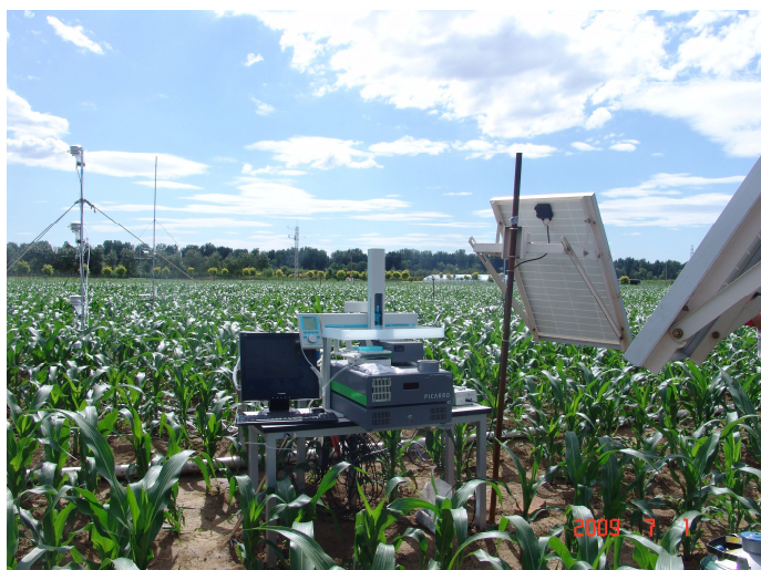
FIG. E-4. Measuring soil evaporation and plant transpiration from a maize field using conventional and isotopic techniques (courtesy of Prof. Xurong Mei).
