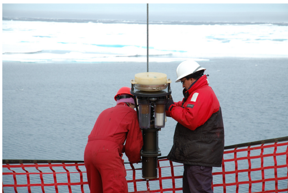
FIG. G-2. Deployment of an in-situ large volume pump to collect particulate material used to measure radionuclides in Arctic waters.
