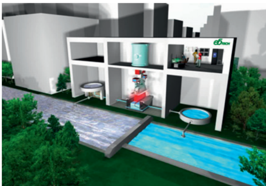
FIG. 2. Electron beam treatment of wastewater (image courtesy of B. Han, Eb-tech).
