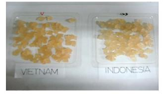
Cassava starch+KOH+AcrylicAcid after irradiaton and dried in preparation of super water absorbent.
