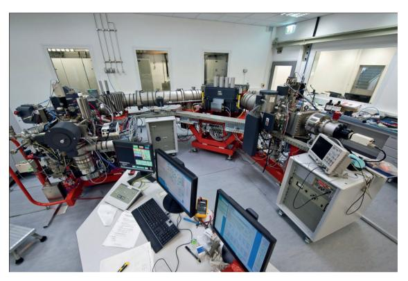
FIG. 3. CAMECA IMS 1280-HR Large Geometry Secondary Ion Mass Spectrometer in service in the Clean Laboratory extension, Seibersdorf.
