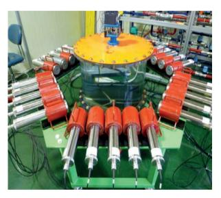
FIG. 3. Industrial single photon emission computed tomography system for the radiotracer visualization of <sup>68</sup>Ga and <sup>137m</sup>Ba from generators.
