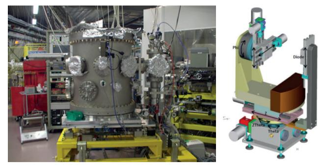
FIG. 4. The UHVC at the Federal Institute of Physics and Technology, Berlin (left), and the seven axis motorized sample manipulator under construction for the Agency's UHVC (right).
