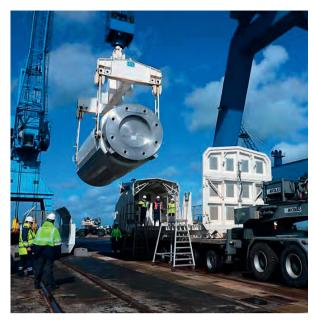
FIG. 3. A transport cask containing radioactive material being loaded for shipment.
