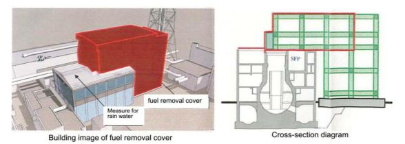
FIG. A-19. Protection cover for the removal of spent fuel from the spent fuel pool at Fukushima Daiichi-4.
