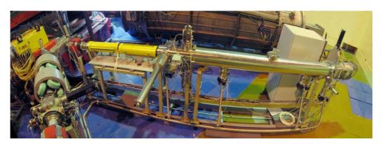
FIG. C-1. Development of a new ion beam line for radiation hardness testing of electronic devices at the U400M cyclotron facility in the Joint Institute for Nuclear Research (Russian Federation).
