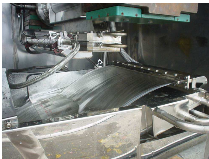
FIG. F-1. Treatment of wastewater using an electron beam accelerator (Photo: EB Tech, Republic of Korea).
