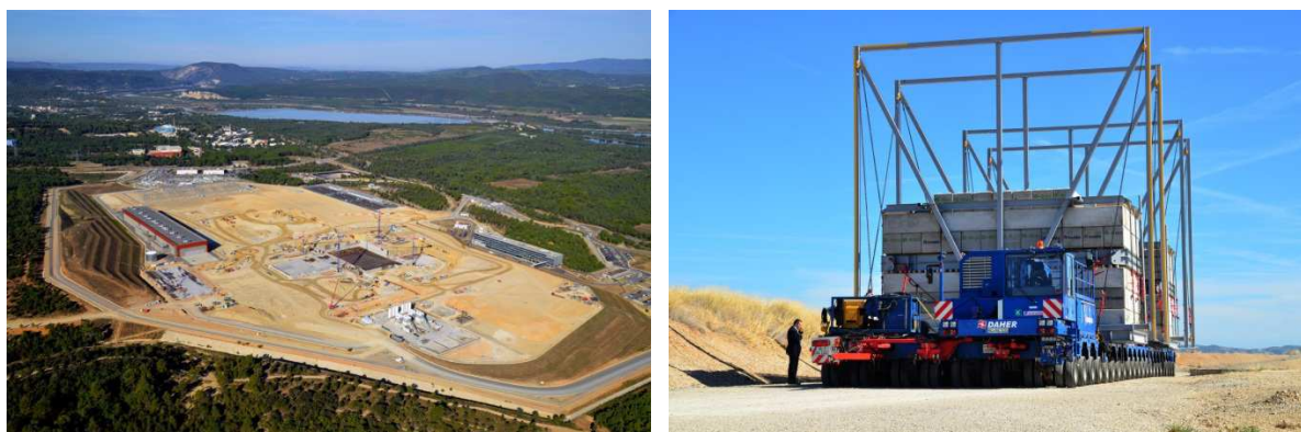
FIG. B-4. The ITER site as of September 2013 (left). The 800-tonne trailer with remote-controlled vehicle, mimicking the weight and dimensions of the largest ITER loads (10 m tall, 33 m long, 9 m wide), travelled at an average speed of 5 km/hour for four consecutive nights to test the 104 km long ‘special itinerary’ (right). (Photos: ITER)
