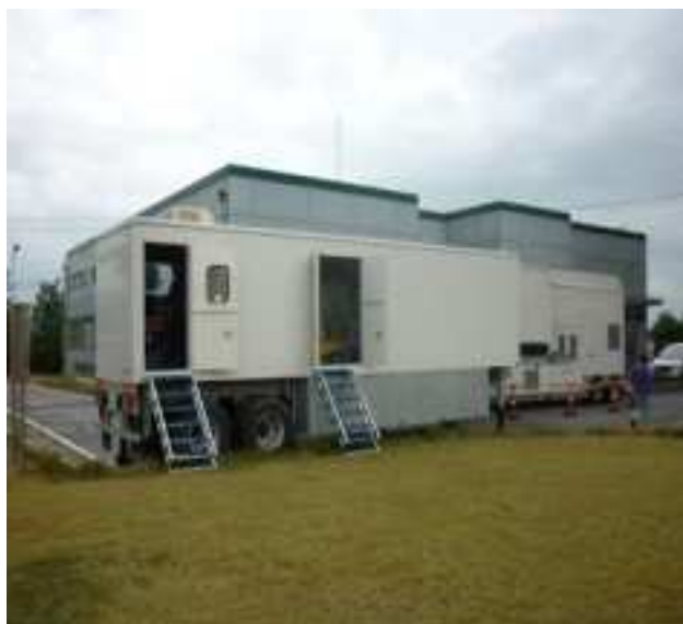
FIG. F-2. A mobile electron beam accelerator installed in sewage treatment plant. (Photo: KAERI)
