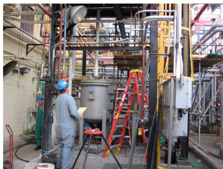
FIG. A-10. New hydrogen fluoride vaporizer, Honeywell Metropolis Works facility, Illinois, USA (Photo: Coverdyn)
