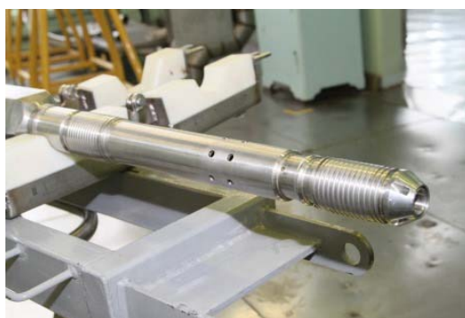
FIG. A-7. TVS-5 fuel assembly, the prototype fuel for the advanced BREST-300 reactor. (Photo: SCC)
