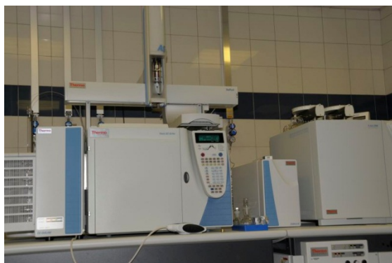
FIG. H-2. Isotope ratio mass spectrometer used to measure stable nitrogen and carbon isotope ratios for studying coastal eutrophication processes
