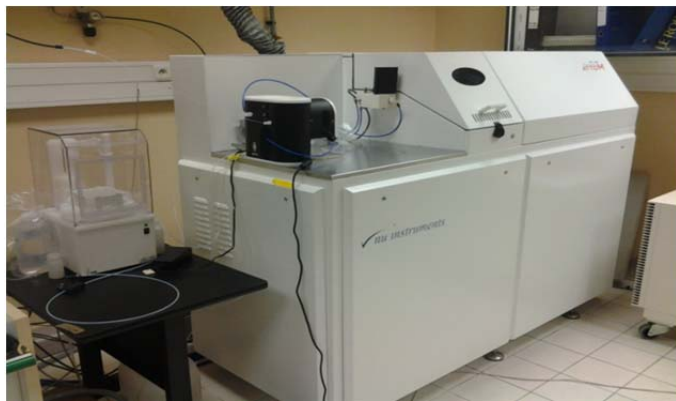
FIG. H-3. High Resolution Inductively coupled plasma mass spectrometer used to analyse stable lead isotopes in environmental samples
