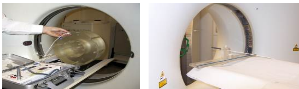
FIG. E-1. Measurement of dose in CT in a standard polymethyl methacrylate body phantom, and in air.
