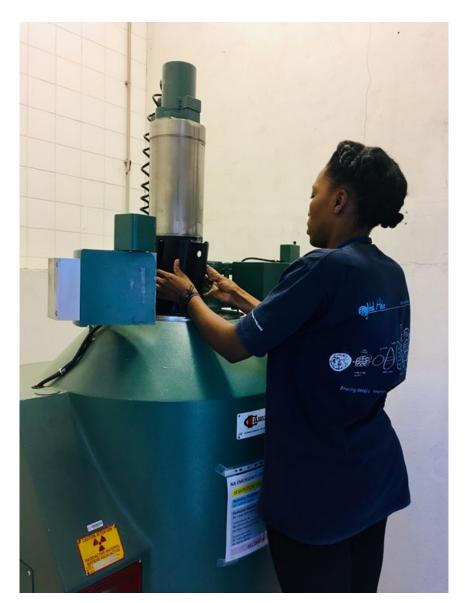
FIG. B.1. Male mosquitoes are loaded into the chamber of a Gammacell 220 unit for sterilization. (Source: IAEA)
