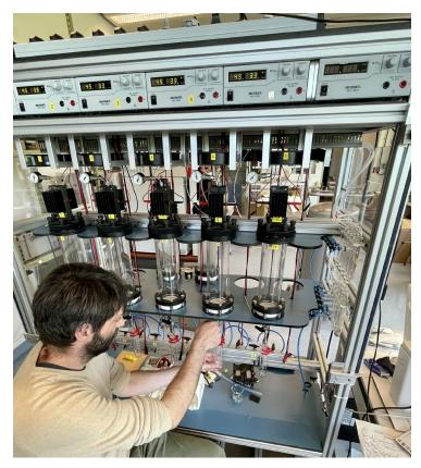
FIG. B.1. New method for tritium enrichment based on permeable electrolytic membrane technology. (Source: IAEA)
