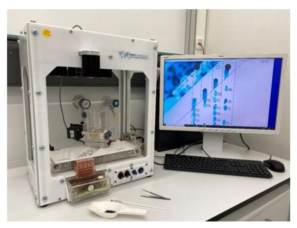
FIG. B.2. The Near Infrared Pupae Sex Sorter for the tsetse fly. (Source: IAEA)
