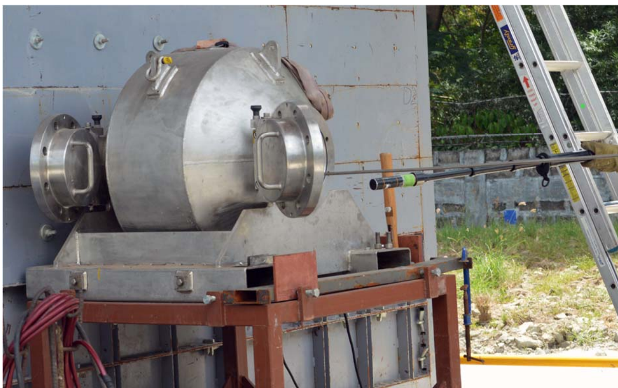
A gamma source removal to a mobile hot cell.
