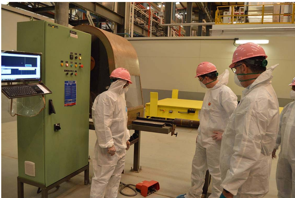
ORPAS reviewers observing a Clearance Assessment System for Pipes assessing a pipe for naturally occurring radioactive material (NORM) residue, Abu Dhabi Oil Refining Company, United Arab Emirates in November 2022.
