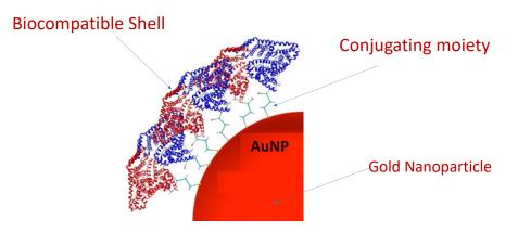
FIG. J.2. Schematics of a conjugated gold (Au) NP used in radiopharmaceutical development. (Graphic: IAEA)
