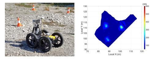
FIG. E.6. An instrumented UGV used in a training workshop at the Nuclear Science and Instrumentation Laboratory in Seibersdorf, Austria (left) together with the obtained radiation map of 'hot zones' (right). CPS stands for counts per second. (Source: IAEA)
