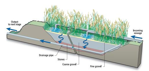
FIG. J.6. A schematic diagram of a constructed wetland. (Source: IAEA, modified graphic from Graphithèque/Adobe Stock)
