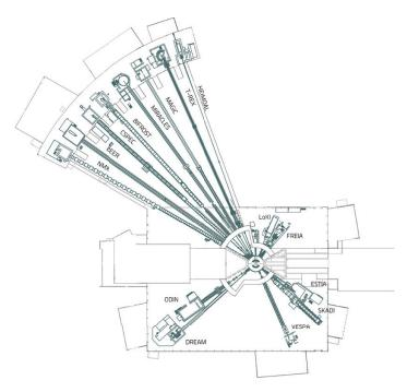
FIG. E.3. A set of neutron scattering and spectroscopy instruments to be offered by the future generation accelerator-based neutron source at ESS. (Source: ESS)
