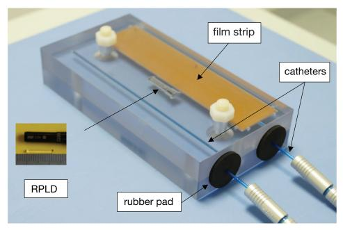
FIG. H.5. A simple, lightweight, cost-effective phantom developed in the Agency's Dosimetry Laboratory and used for brachytherapy audits (RPLD — radiophotoluminescent dosimeter). (Photo: IAEA)
