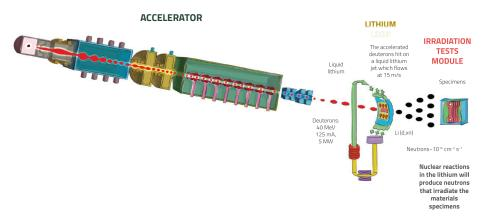
FIG. E.4. Schematics of the IFMIF-DONES facility based on a high-power deuteron accelerator, liquid lithium target loop for high energy neutron production and a material irradiation tests module. (Source: IFMIF-DONES)
