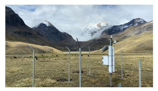
FIG. I.4: A CRNS installed in the high altitude Andean Bolivian wetlands to study their role in buffering water under climate change. (Photo: T. Franz, University of Nebraska–Lincoln)
