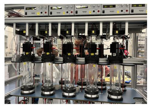
FIG. K.2. A front view of the Agency's PEM tritium system, consisting of ten electrolytic cells running a set of reference samples to test accuracy and precision. (Photo: IAEA)
