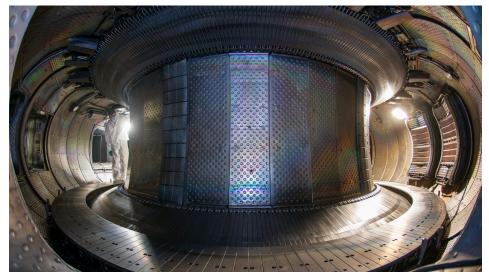
FIG. D.5. WEST tokamak equipped with its actively cooled tungsten diverter. (Source: CEA)
