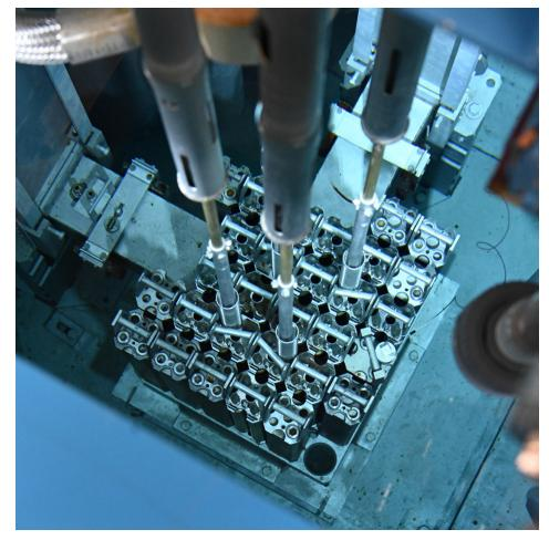
FIG. E.2. A view of NRAD's reactor core with its internal equipment for materials research at the INL. (Source: INL)
