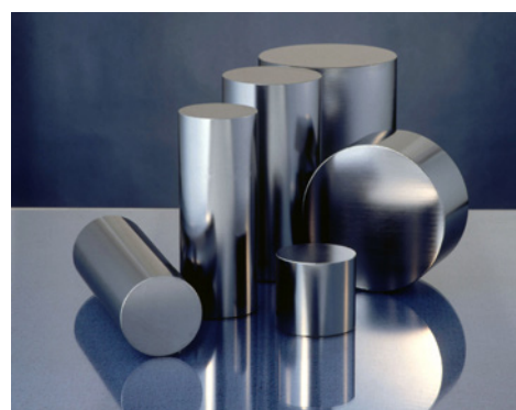
FIG. E.5. Silicon ingots of different dimensions— one of the irradiation products from the OPAL research reactor in Australia. (Source: Australian Nuclear Science and Technology Organisation)
