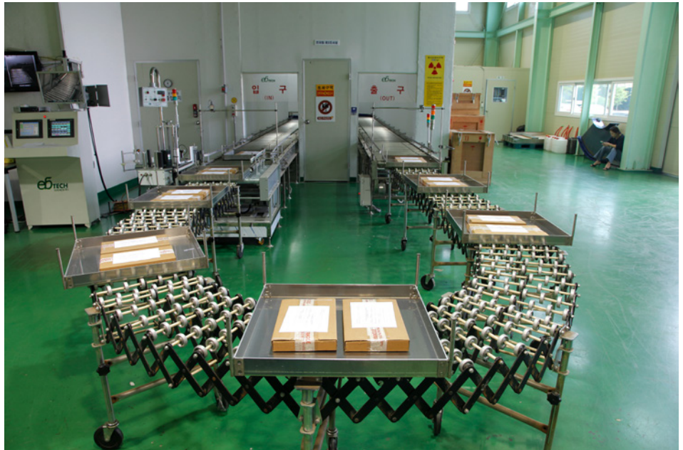
FIG. K.3. Electron beams are currently used for industrial purposes in 40 Member States. Here, semiconductors are irradiated with a 10 MeV (20 kW) electron beam system in a private enterprise in Daejeon, Republic of Korea. (Source: IAEA)
