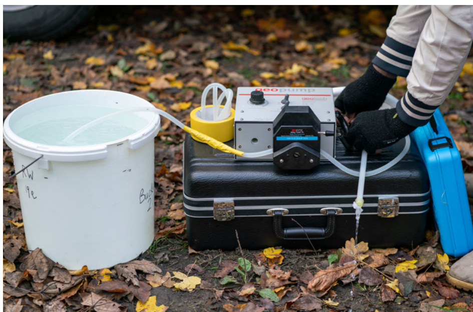
FIG. L.2. Collection and concentration of sulphur-35 in the field from groundwater samples using portable resin columns. (Photo: IAEA)
