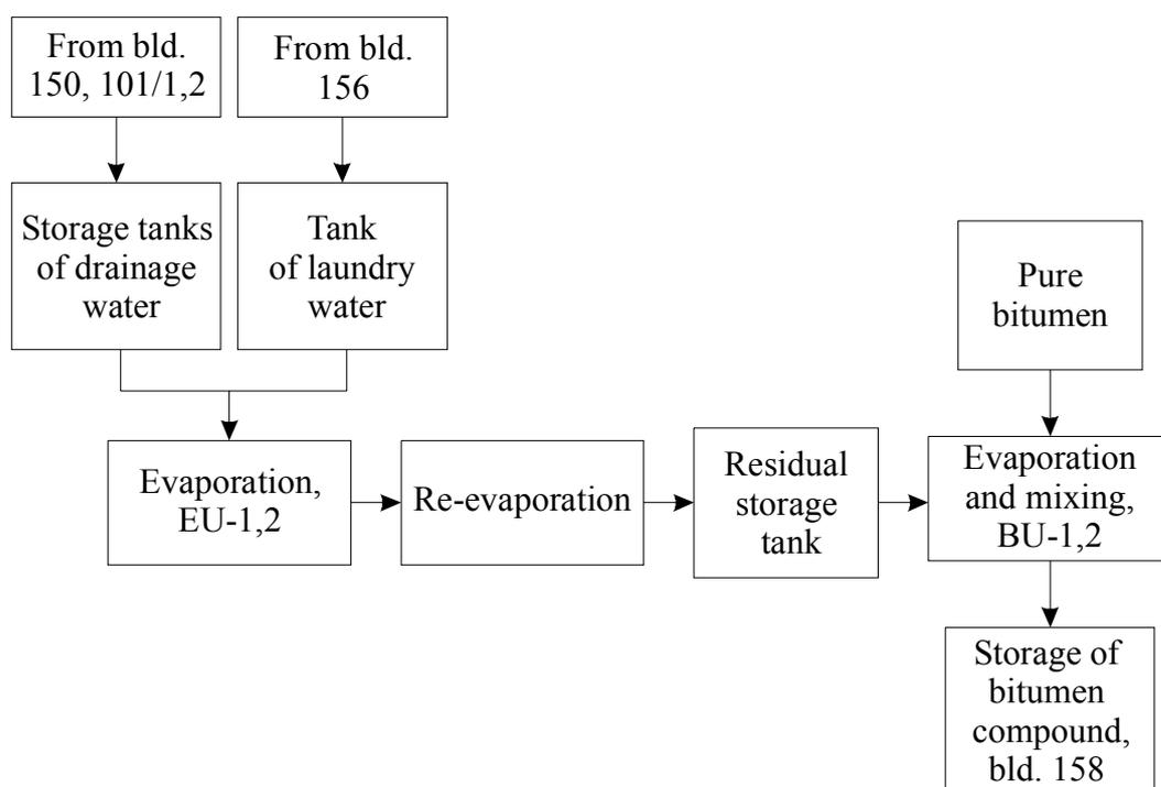
**Figure D-2. The process of the collection of the liquid radioactive waste and the following bituminisation at Ignalina NPP**
