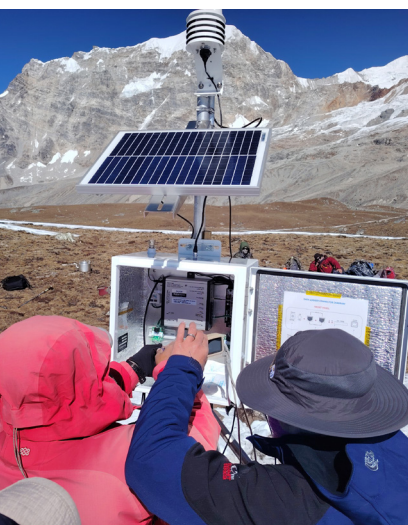
The cosmic ray neutron sensor was assembled on the Yala Glacier in Nepal after a six-day trek.
