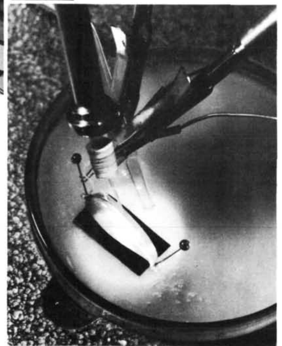
Enlargement of frog muscle with micro-electrode inserted
