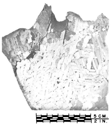
Crystal size in the Bogou meteorite indicates that it was originally part of a much larger body and that cooling was very slow. Much of the surface was burned or melted away after entering the atmosphere at about 125 000 miles an hour.
