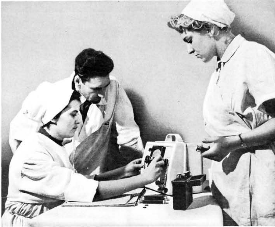
Many hospitals in USSR use radioactive isotopes for diagnosis and therapy. For the safety of personnel individual dosimeters, here being checked after use, are worn by medical staff.
