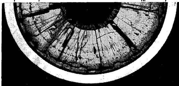
Radial analysis of fission products by Gamma ray spectrometry.
