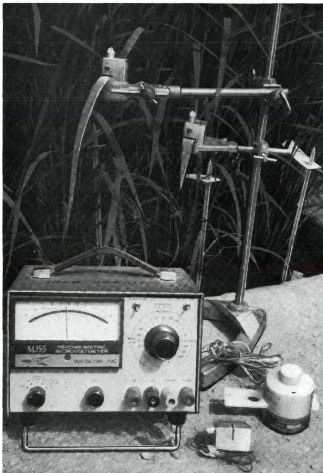
A psychrometer at work on plant leaf and in soil.
