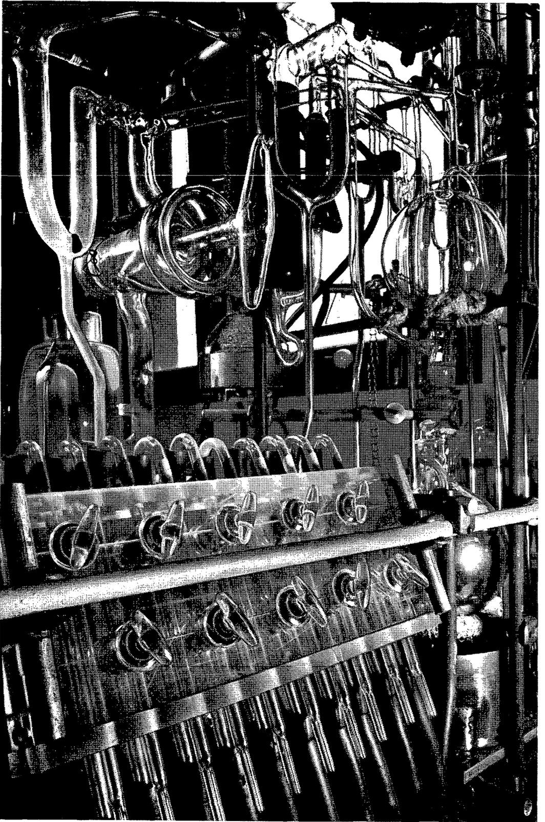
Laboratory equipment used to extract gases from metals at the Saclay Atomic Energy Centre.
