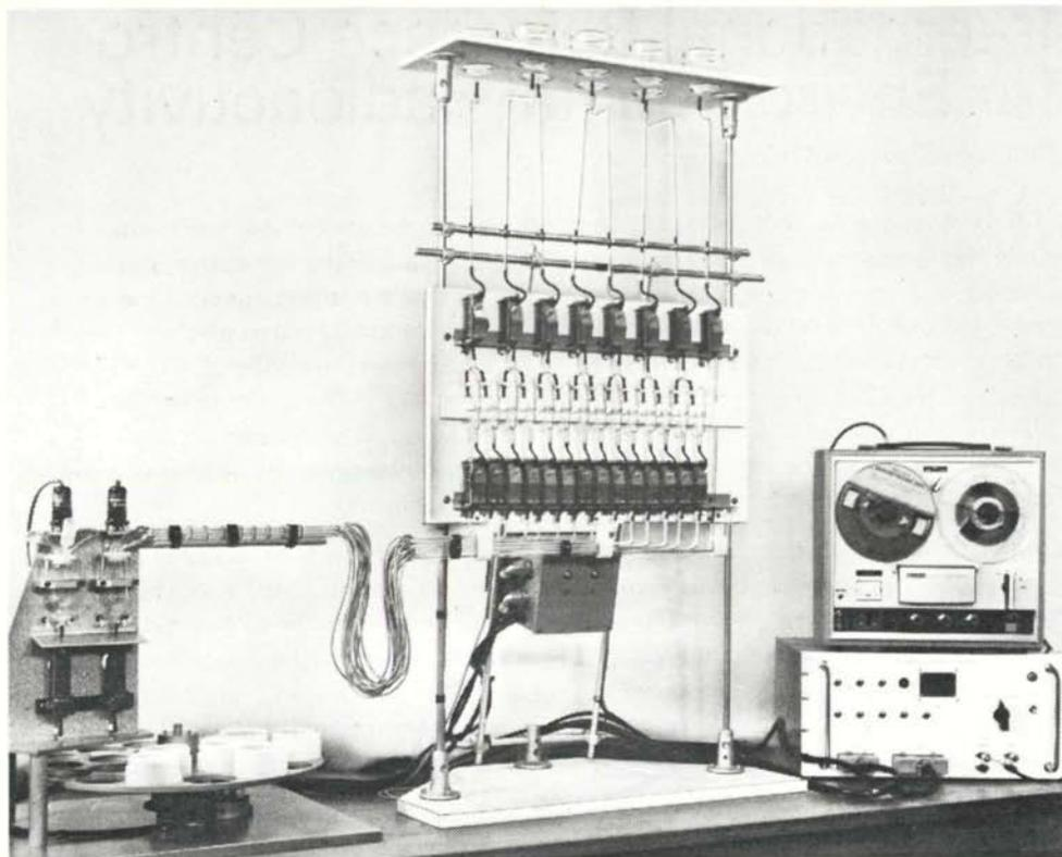
Automated radiochemical separator for the determination of cadmium, chromium, copper, molybdenum and zinc by neutron activation analysis. The samples, in a suitably oxidised form, are introduced into the separator in a dilute sulphuric acid medium. The radionuclides of interest are separated into three chemical fractions suitable for subsequent measurement with a NaI(Tl) or Ge(Li) detector. Two samples are processed concurrently in about 30 minutes – UKEA Aldermaston
