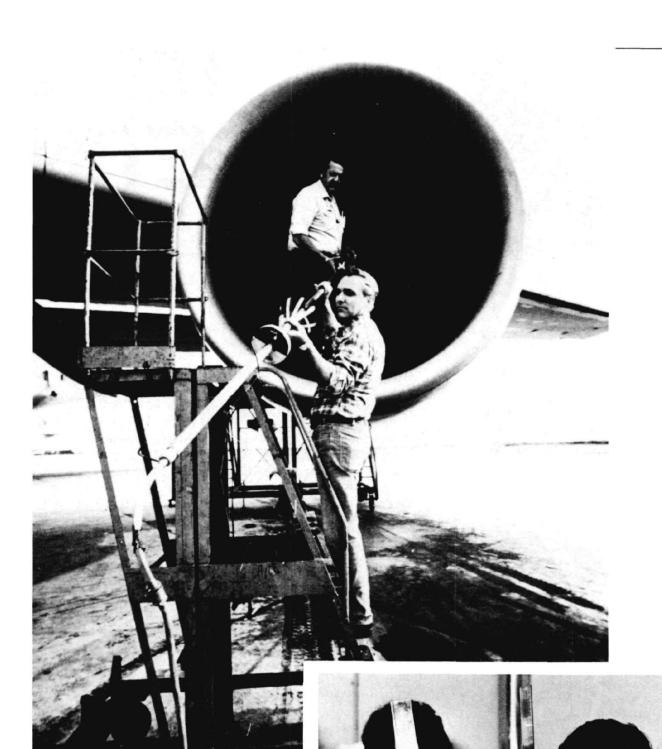
Among typical uses of commonly transported radionuclides are plant and crop research in agriculture, and quality-control inspections in aircraft and other industrial machinery. Top photo shows gamma radiography equipment being used to check engine interiors of a passenger jet. (Credit: Tech/Ops)
