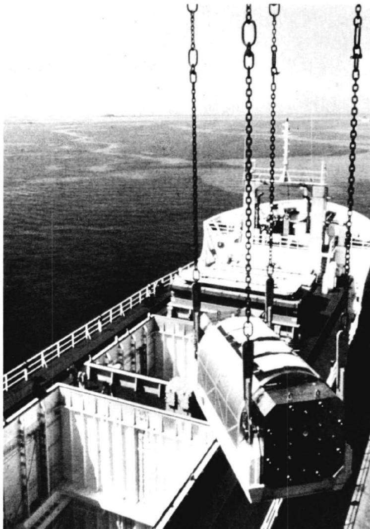
Contained inside a forged steel cask called a TN-12 package, irradiated fuel is lowered to fit into a specially-designed compartment for safe sea shipment. (Credit: Transnucléaire)
