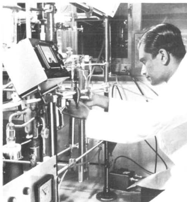
The 1000th IAEA fellowship was awarded to Dr. P.P.G.L. Siriwardene, of the University of Ceylon, Colombo, for training at the UKAEA Isotope School at the Wantage Research Laboratory in Berkshire, UK. Picture shows Dr. Siriwardene operating a vacuum apparatus used in the counting of tritium (Photo UKAEA)
