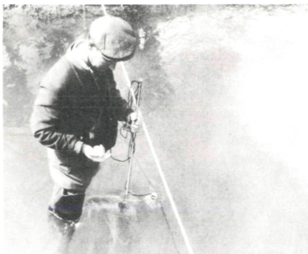
Measuring flow rate of water in UN Special Fund ground water project in Greece (Photo: Greek Atomic Energy Commission)
