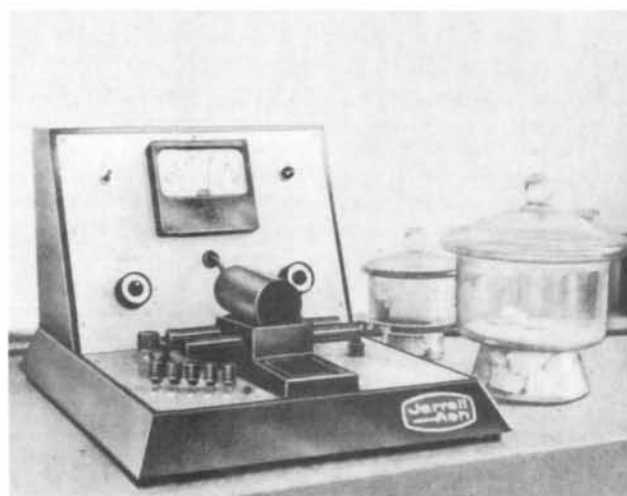
A fluorimeter supplied by IAEA installed in the laboratory. The instrument is used for the determination of uranium by fluorescence methods
