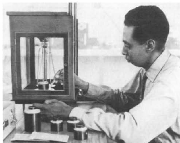
A Ceylonese geologist, Mr. Stephen Kumarapeli, weighing samples for radiometric assay
