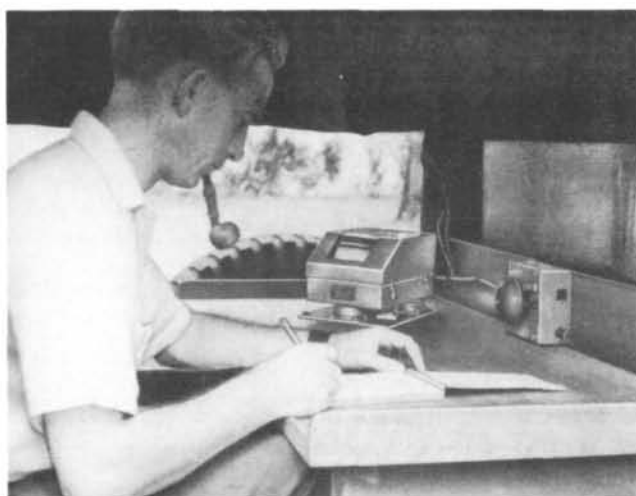
The IAEA expert operating the equipment for car-borne surveys. The recorder and alarm unit can be seen fitted to a table installed in the rear of the vehicle
