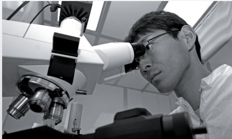
A technician at the Safeguards Analytical Laboratory in Seibersdorf examining uranium particles under an optical microscope.
