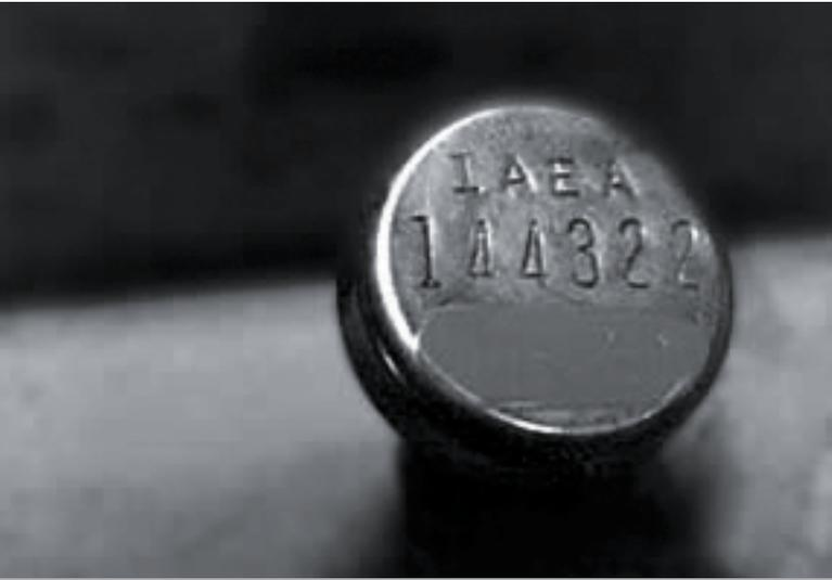
Metallic seals like the one in the picture are commonly used by safeguards inspectors. The seals provide important evidence of any unauthorized attempt to gain access to the secured material.
