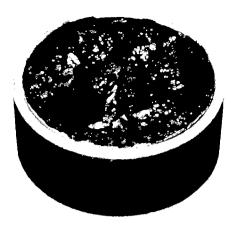
Photograph of a glass product containing radioactive waste. (From paper by M.N. Elliot, R. Gayler, J.R. Grover and W.H. Hardwick)
