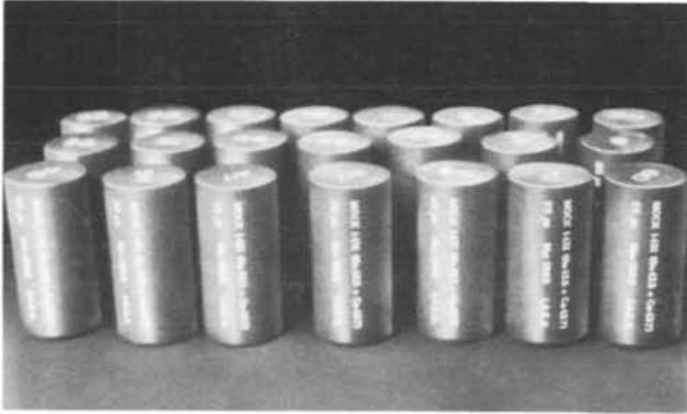
As part of its efforts to develop the medical uses of radioisotopes, the Agency has undertaken a programme for the calibration and standardization of measurements of radioiodine uptake by the thyroid gland. "Mock" radioiodine sources (a substance with radiation characteristics nearly identical to those of iodine-131 but with a much longer half-life) are used as standards in this work. Picture shows these sources (containing barium-133 and caesium-137) ready for despatch
