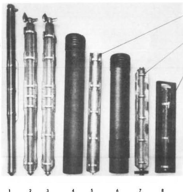
Some of the magnox fuel elements manufactured by the UK Atomic Energy Authority. 1. Calder Hall element; 2. Latina element; 3. Bradwell Mk III element; 4. Tokai-Mura graphite sleeve; 5. Tokai-Mura element; 6. Hunterston sleeve; 7. Hunterston element; 8. Berkeley Mk. 1B. (Picture reproduced from paper by C. Allday)
