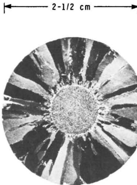
Cross-section of a uranium dioxide cylinder.
