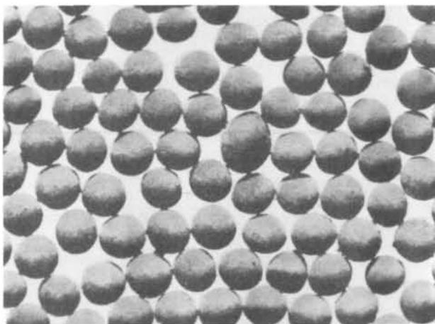
These three photographs, taken from the paper by H. Lloyd, show the progressive rounding of uranium dioxide granules by gyration. The picture on top shows the granules before being subjected to the gyration process, the one in the middle was taken after four hours' gyration and the one at bottom after nine hours' gyration.
