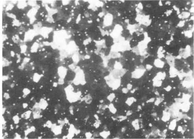
The microstructure of a hot-compressed solid solution of zirconium carbide and uranium carbide. (Picture reproduced from a paper by R.B. Kotelnikov and others)
