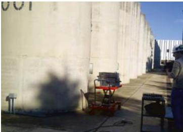
PUI funds are also being used to support research on the very long term storage performance of spent nuclear fuel and related storage system components. This also includes research into the long term integrity of dry storage concrete systems. Using an experimental setup of LaBr3 and NaI(TI) gamma detectors, experts check the confinement integrity of the spent fuel and the structural integrity of the reinforced concrete silos at Embalse NPP's dry storage, Argentina. (Photo: CNEA/NA-SA)
