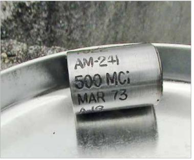
Sealed radioactive sources or "sealed sources" are radioactive materials that have been isolated/sealed in metal capsules like this one. Sealed sources are used in many fields, such as medical diagnostics and treatment, to control industrial processes, and to sterilize food and medical products.
