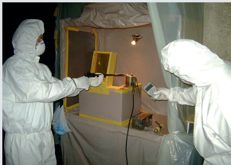
Verifying the radioactivity level of a capsule containing conditioned caesium-137 sources. (Photo: J. Balla/IAEA)
