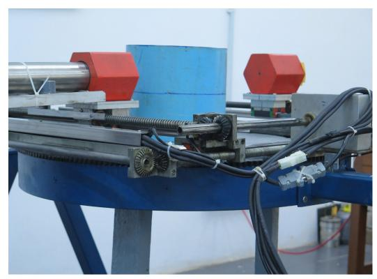
This NDT device emits radiation from the radioactive source (left). The radioactive particles react with the substance in the light blue pipe in the middle. The detector on the other side of the pipe measures radiation. This measurement provides information about the quality and quantity of the material going through the pipe. (Photo: M. Gaspar/IAEA)
