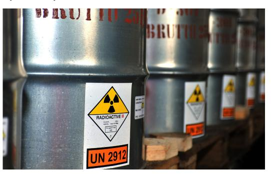
Yellowcake is packed in special, tightly sealed steel drums similar in size to oil barrels. Each weighs no more than 350 kilogrammes when full. (Photo: D. Calma/IAEA)
