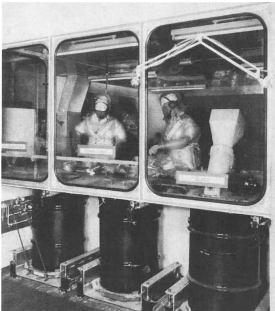
Sorting of radioactive wastes inside a sealed area, by men in pressurized suits. (From paper by R.H. Burns and others)
