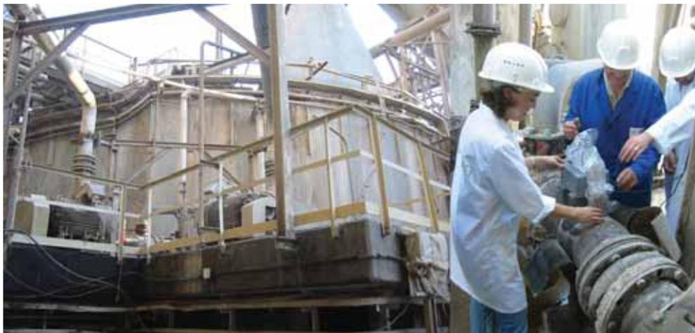
FIG. 3. Optimizing phosphoric acid production using radiotracer techniques at a plant in Tunisia.
