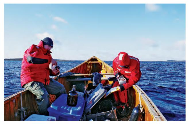
FIG. 1. Sampling in the St. Lawrence River as part of an isotope monitoring programme in Canada. (Photograph courtesy of J.-F. Hélie.)
