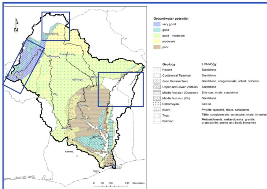
Figure 7: Geological map and groundwater potential of the Volta Basin, showing the three studied sectors (in Martin, 2006)
