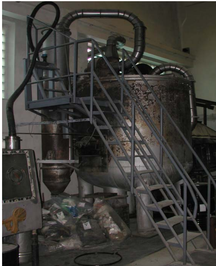
Incinerator for solid radioactive waste contaminated with U-nat
