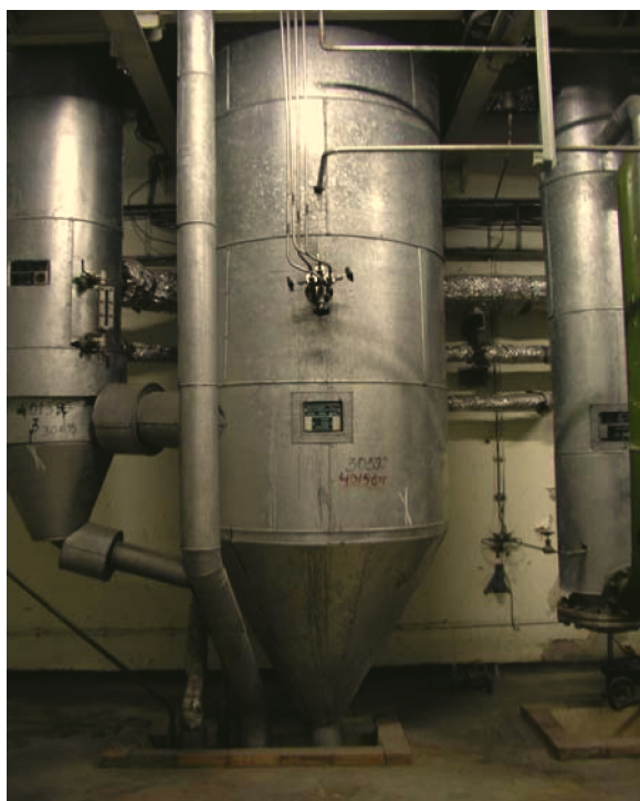
Evaporator for treatment of low - active \beta - \gamma liquid wastes
