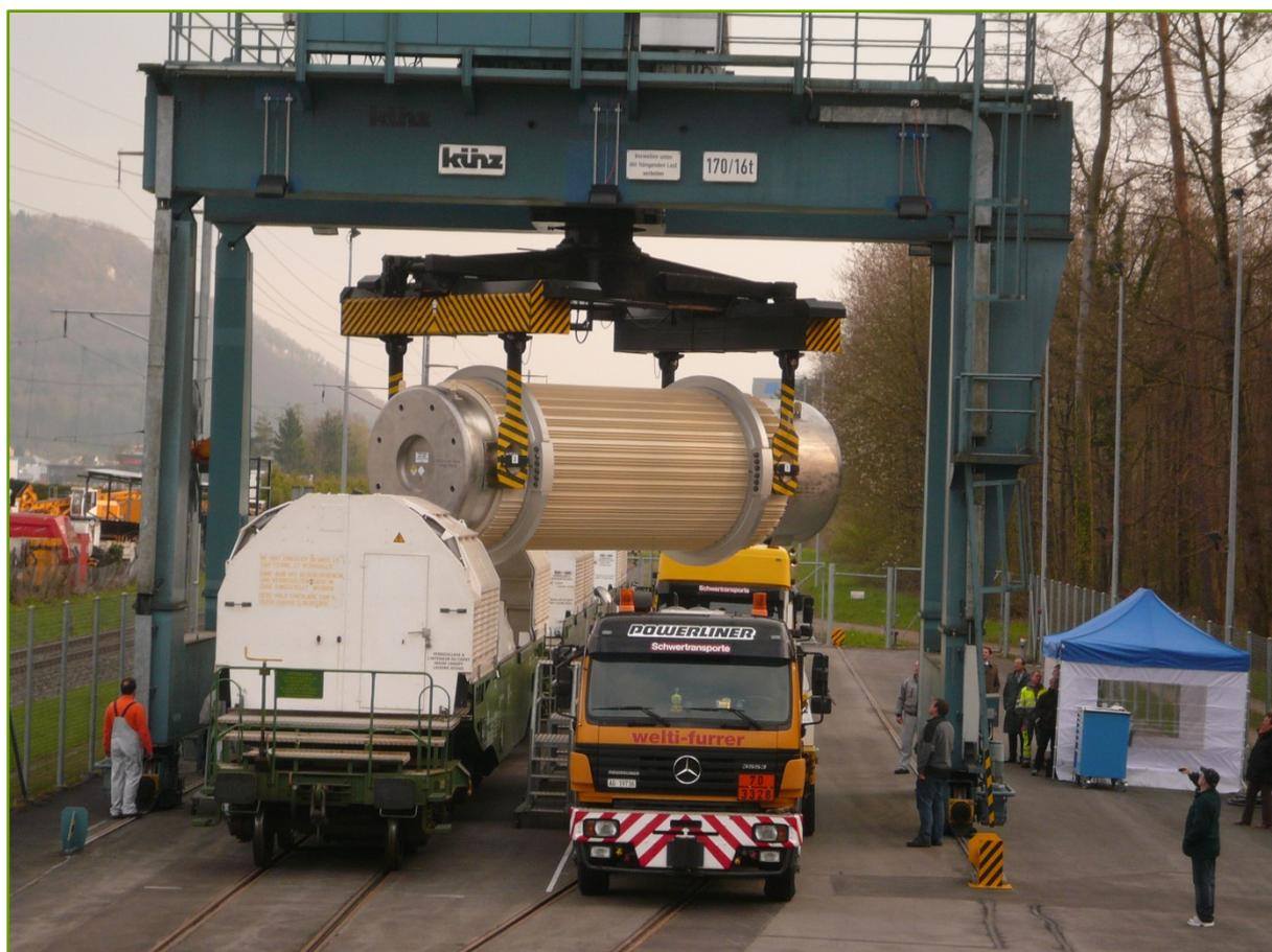
Figure 14: Arrival of radioactive waste returned from reprocessing in the transbordement facility of Zwiilag (Photo ENSI)
